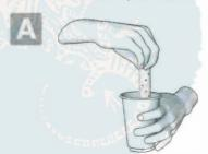
Remove HC1D HydraCell from plastic sealing. Immerse cell fully in water for 15 seconds.
