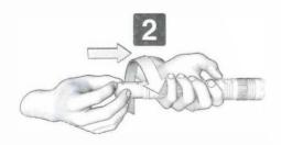
Cell fits snugly in AguaFlash barrel. Use a twisting motion to fully insert activated cell, confirming cell is properly seated. Replace rear section, making sure rear section is properly threaded on.
